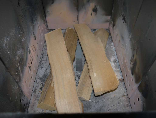
Figure 7 Basic layer of wood during heat-up
