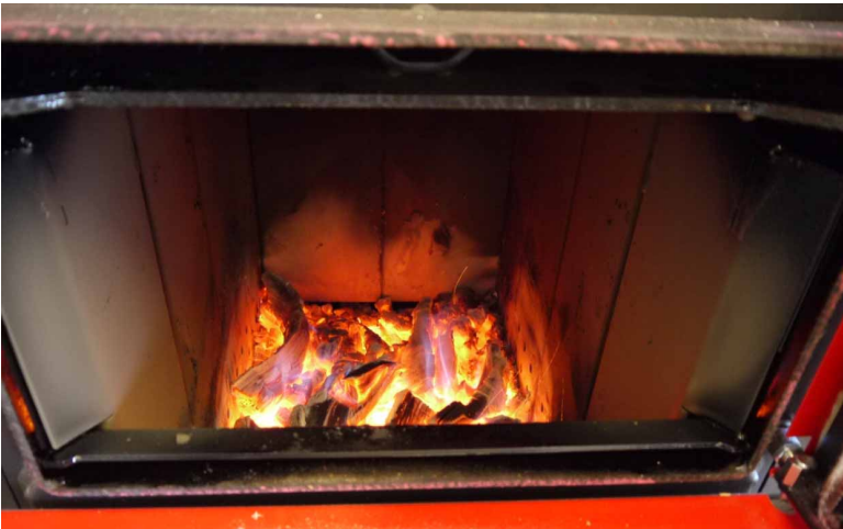
Figure 13 Height of the live coals suitable for stoking.
