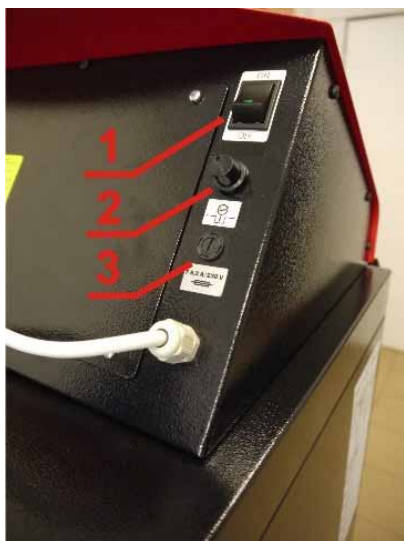
Figure 17 1 – main switch, 2 – emergency thermostat, 3 – fuse (F6, 3 A)
