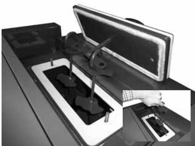
Example of removal of decelerators from the tube exchanger (tube plate) before thorough cleaning
